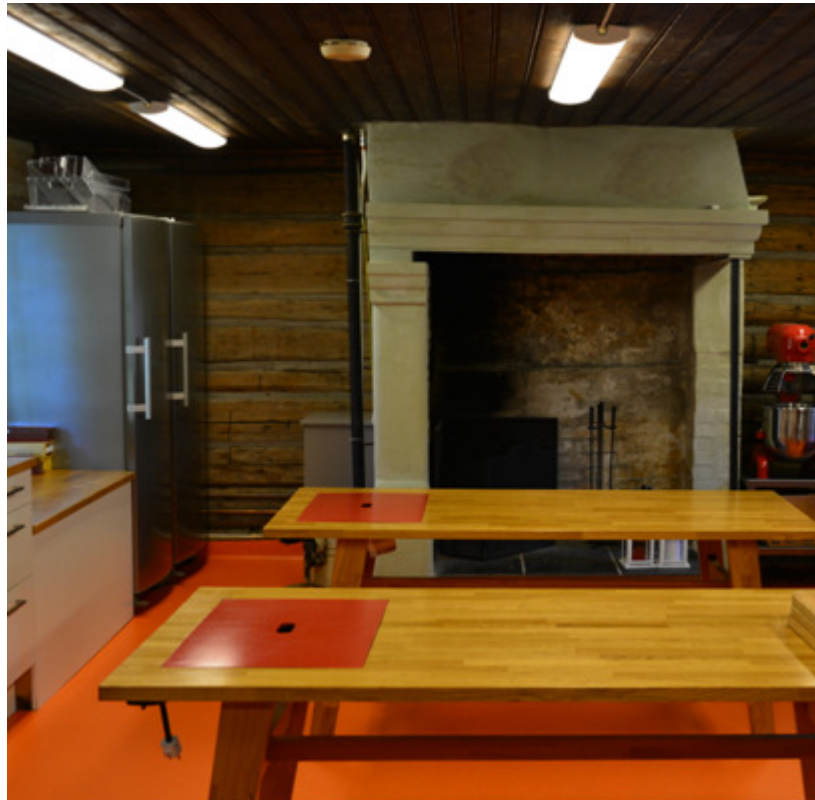
A work bench designed for the size of 10-12 year old children with a safe (covered) hot-plate.
